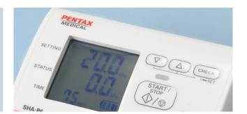
The SHA-P6 Auto Leakage Tester is specifically designed for use with PENTAX Medical flexible endoscopes to avoid costly service interventions associated with undetected leaks.
