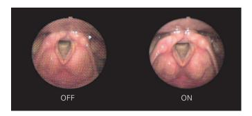
Clear image: Anti-moiré filter to sharpen the fibre endoscope image
